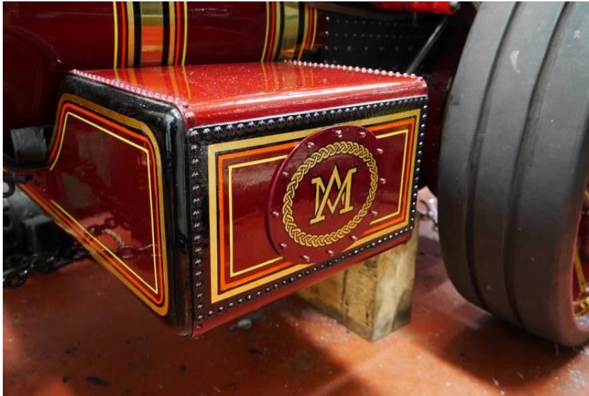
Figure 3 Lining on the belly tank
