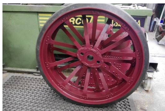
Figure 2 Rear wheel awaiting the top coats
